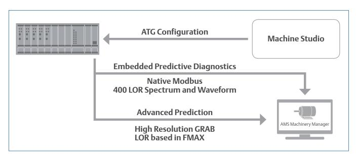
AMS 6500 ATG provides new communication protocol with embedded OPC UA technology.
